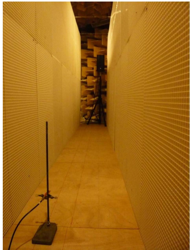
FIG. 7. (Color online) Photograph showing the setup of the indoor experiment conducted in an anechoic chamber.
